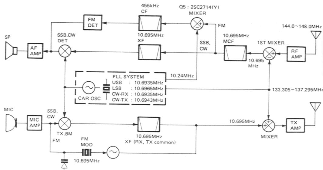
Fig. 1 Frequency configuration
