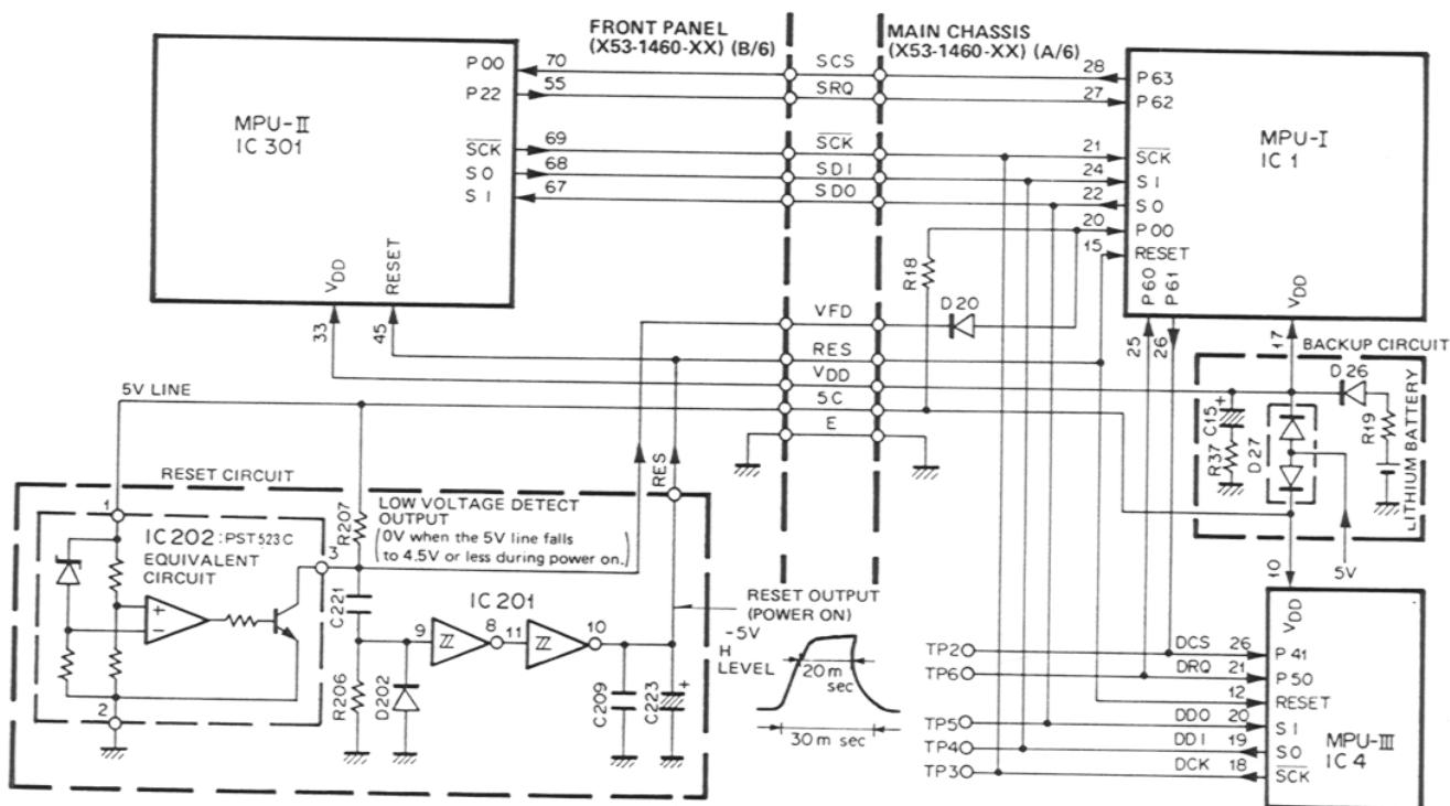
Fig. 9 Interface between MPUs and reset backup circuit
