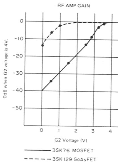
Fig. 2 AGC attenuation comparison
