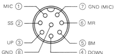
Fig. 12 MIC terminals (view from front panel side)
