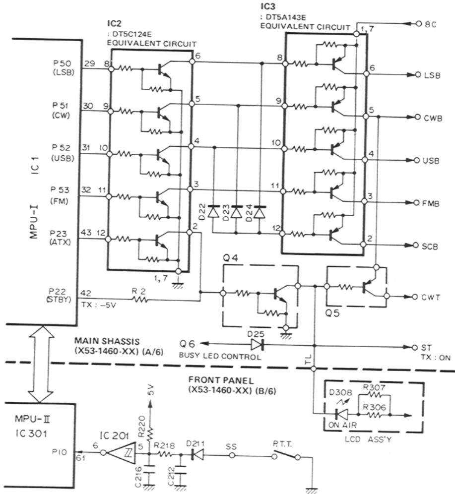
Fig. 11 MODE voltage switching and standby circuit
