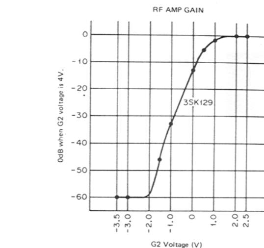
Fig. 4 AGC attenuation comparison
