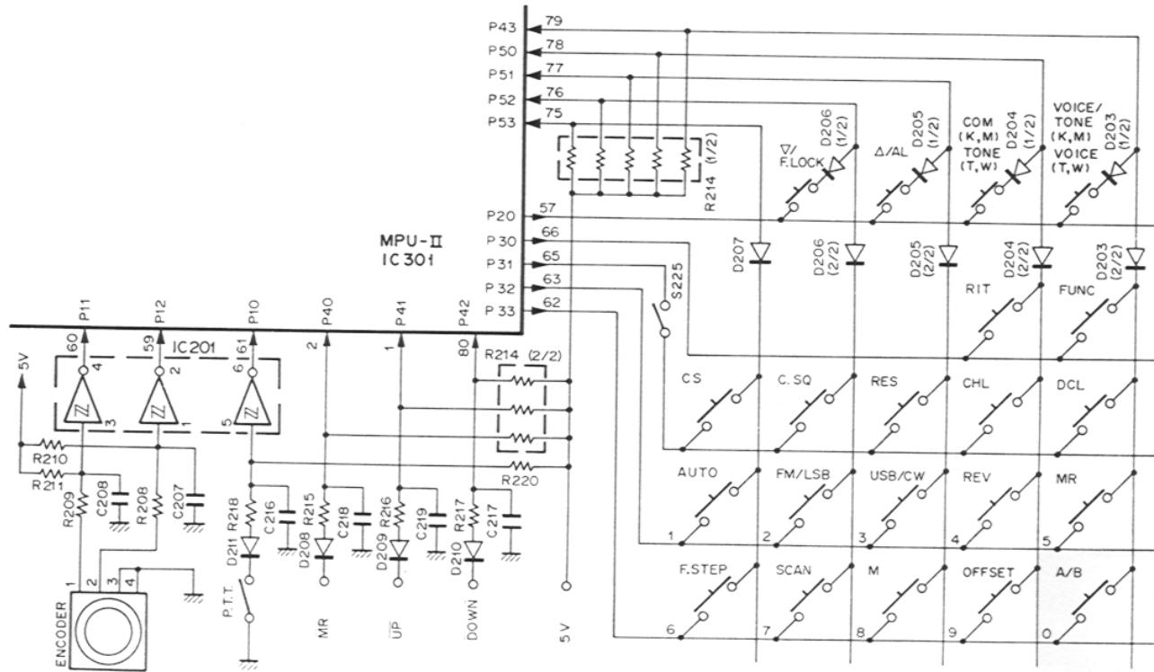
Fig. 10 Key, switch and encoder input circuit
